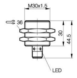
Inductive Sensors BES 516-359-E5-Y-S 4 M30x1.5 x 44.5 normally-open Sn=10mm shielded
